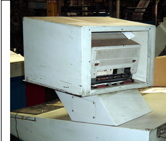
Rear view of one of the press control consoles at Quebecor World's Riverside plant showing the original Intecolor 3810 terminal prior to removal and replacement.
