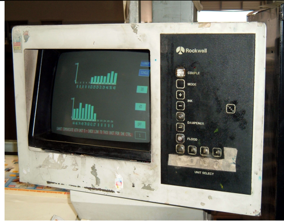
Front view of the press control console showing the original Intecolor 3810 terminal ready for removal from the rear.
